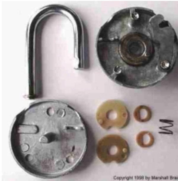
Figure 1.5.1 Internals of a Combination Lock [How] and Figure 1.5.2 Master Lock [Master]
